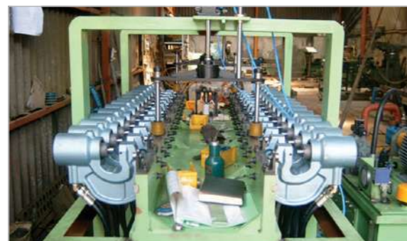
An application for aluminium angle punching with 26 sets of EHPU-2416
